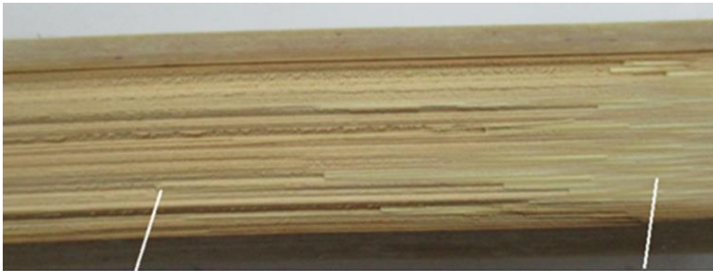
Produced surface due skinning failure (bending) Good produced surface (no bending exists)
